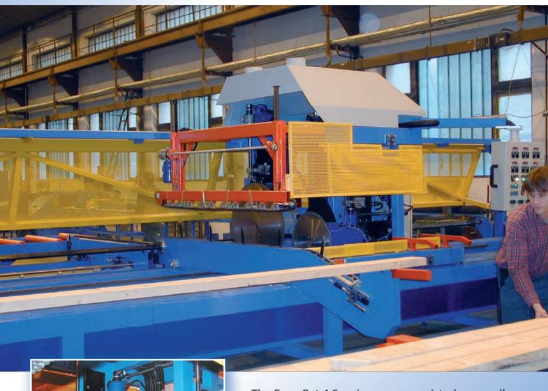
The Easy-Cut 4 Saw is a power-assisted, manually set up component saw, where all axis positions are set up using push-button control and LCD read-outs at two control panels.
