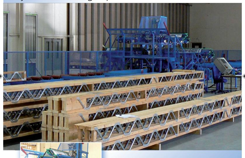
The ReVolution has a unique and patented vertical pressing station with CNC controlled positioning of the Posi-Strut<sup>™</sup> webs ensuring precise and accurate placement every time and eliminating lengthy setting up procedures. Capable of over 1500m in a single shift.
