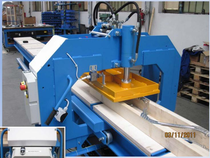
The manual Strut-Runner allows the manufacture of any type of parallel chord truss up to 550 mm in height. (PS8 up to PS16).
