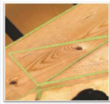
The Virtek Trussline Laser projection system reduces set up times, errors and increases productivity.
